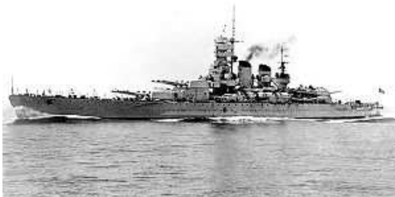
The "Vittorio Veneto" with her 3 turrets each mounting three 15in guns, joins the Regia Marina. Italy is staking her claim to the Mediterranean
